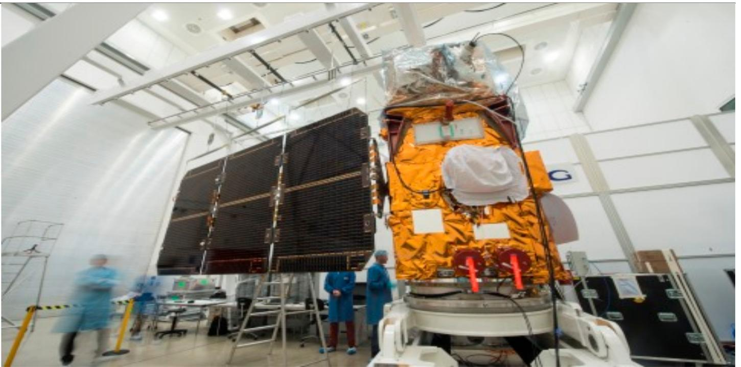
Once in space, Sentinel-2A will open its solar wing to generate the power it needs to carry out the task of monitoring Earth's vegetation. Engineers have recently made sure this move is well rehearsed before the satellite is packed up and shipped to the launch site.
